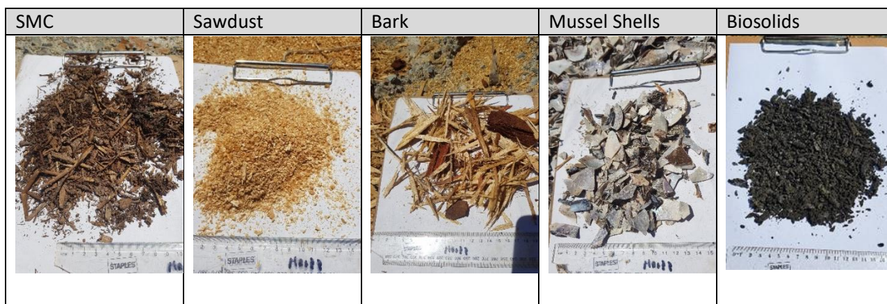
Figure 4.3-9: Photographs of materials used in bioreactors with a 30cm ruler for scale.
