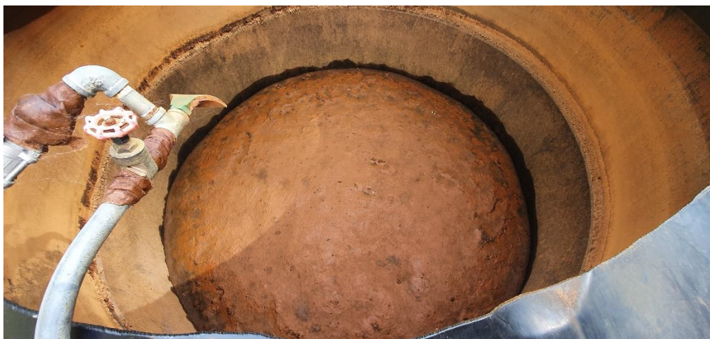
Figure 10: Photographs of arsenic speciation and the vertical flow reactor after being drained. A: Sample preparation for arsenic speciation at the CRL Lab in Christchurch; B: Prepped samples for the arsenic speciation; and C: The vertical flow reactor after being drained for the second time prior to sludge sampling.
