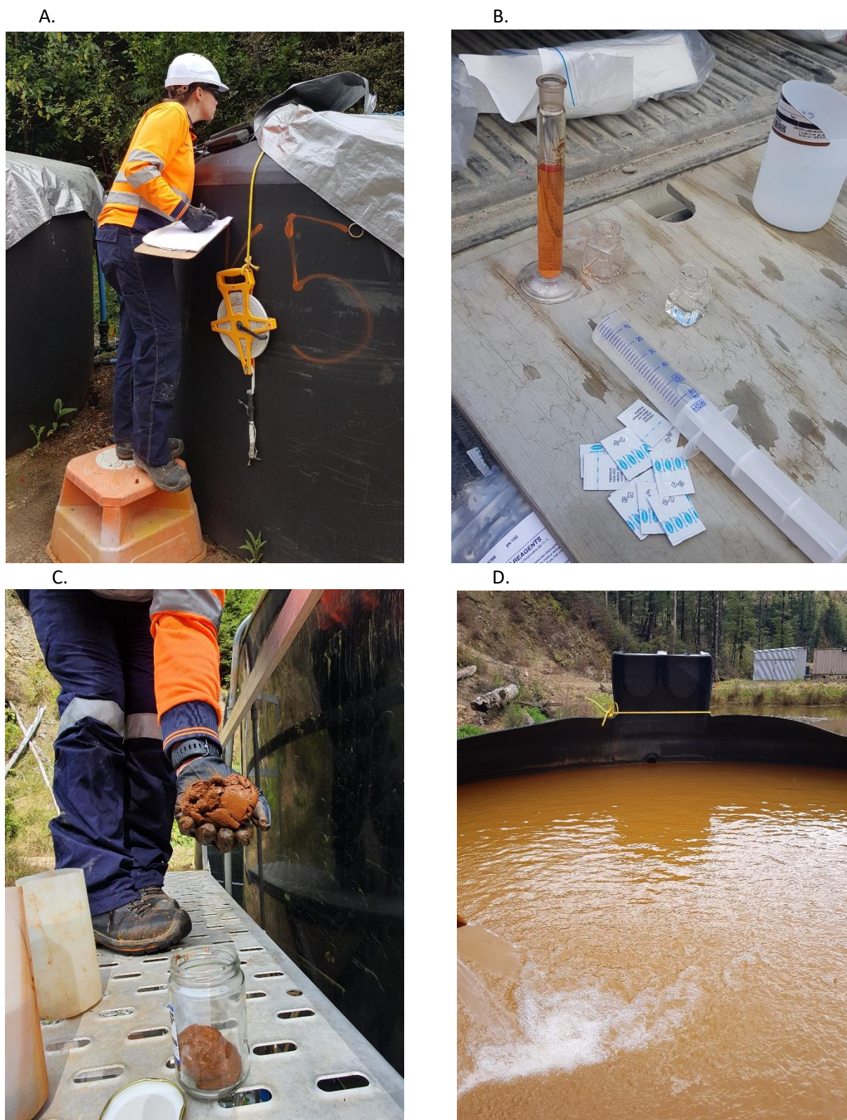
Figure 11: Photographs of the bioreactor field measurements and of the vertical flow reactor and its sludge. A: Physico chemical field measurements being undertaken on tank 5; B: Ferrous iron field measurements with the portable spectrometer; C: Sludge from the second round of sludge sampling from the vertical flow reactor; and D: the vertical flow reactor overtopping.
