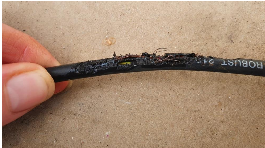
Figure 6.2- 3: Photograph showing damage to the small temperature control middle probe cable due to rat gnawing
