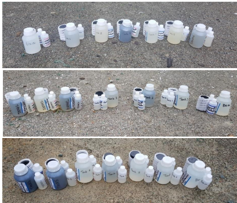
Figure 6.2- 5: Series of photographs of samples taken on different occasions during the 2-year operation of these systems. Note: top photo shows, from left to right, Influent, tank1, tank 2 ,..., tank 6. Bottom two photos show tank 6, tank5, tank4, ... , influent.
