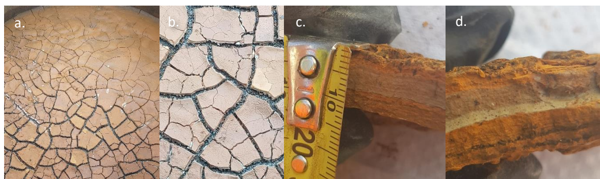
Figure 5.6- 8: Photographs of iron precipitate sludge from first draining event after 12 days of drying. a) Sludge in tank starting to crack as it dries, b) Zoomed in image of cracked sludge in-situ, c) Caked sludge removed from tank showing dried thickness d) Caked sludge removed from tank showing laminations of light sediment.
