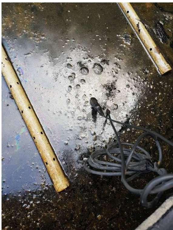
Figure 8: Photographs of the bioreactor sampling and field measurements. A: Sulphide field measurements with the portable spectrometer; B: Sulphide field measurements with the portable spectrometer; C: Probes in the free water in the top of the bioreactors measuring physico-chemical properties; and D: Effluent from the tanks where the samples are taken.
