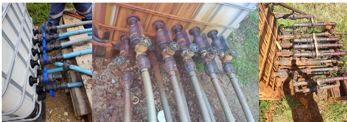
Figure 4.3-8: Evolution of Valves. From Left: ball valve, ball valve with gate valve, and ball valve with gate valve and flushing line.
